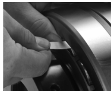
Fig. 18. Measure RIC before installation.
