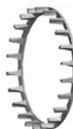
Fig. 7. YMD Split, machined-brass, land-riding, finger-type cage.
