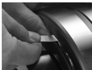
Fig. 14. Measure RIC before installation.
